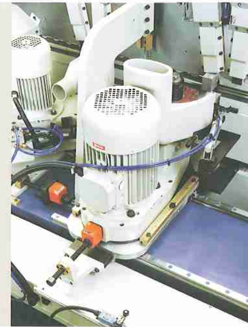
PROFILING UNIT "J-2" with back-up blocks and pneumatic chip-breaker
